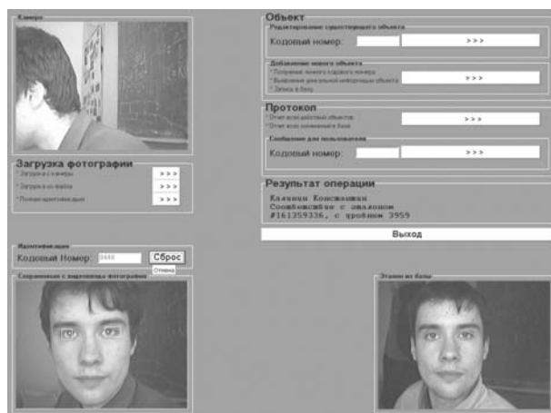
Fig. 1. An example of the subsystem "Identification sector" work. The screen is divided into 4 regions: the upper left-hand region is on line video-input window; the upper right-hand region is a service region available to the "Administrator" only; the lower left- and right-hand regions show the current and template images correspondingly.
