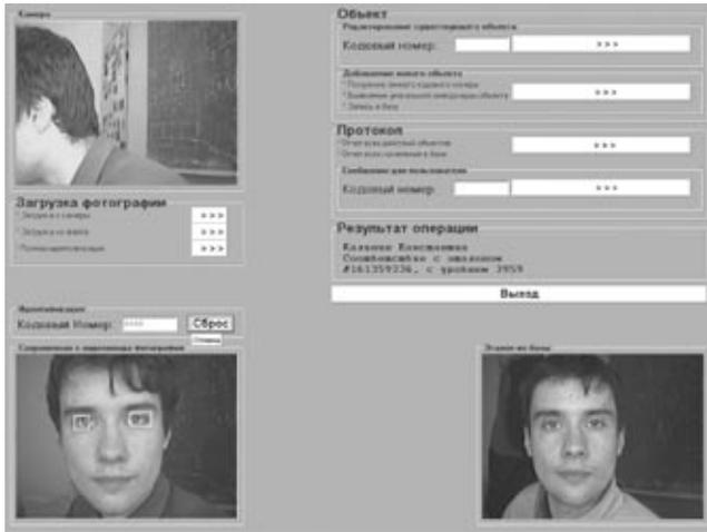
**Fig. 1.** Operation of the Identification Sector subsystem. The screen is divided into four regions: the top left region is the online video-input window, the top right region is a service region available for the Administrator only, and the bottom left and right regions show the current and template images, respectively.
