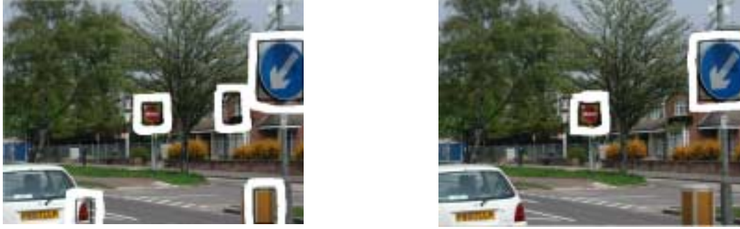
Fig. 4. The initial results of segmentation (a) (regions marked by white contours); rejection of false regions after the recognition stage (b).
